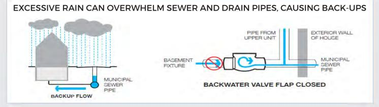
During a rainfall or sewer backup event, the backwater valve closes to block sanitary sewage from entering your basement fixtures. Please be aware that closed valves also prevent basement wastewater from exiting into municipal sewer pipes.
