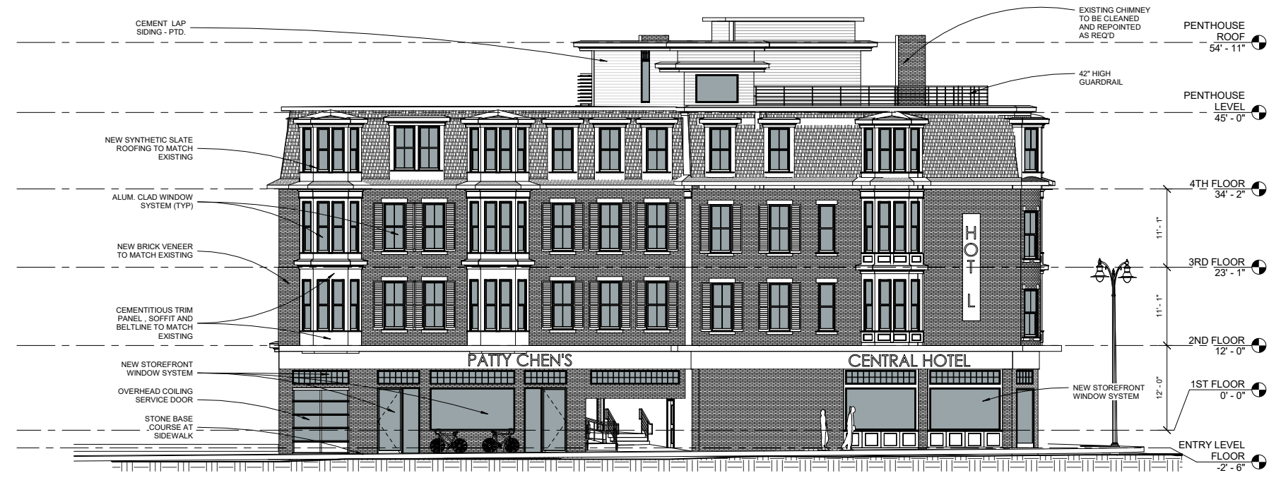
② FRONT ELEVATION - COLUMBIA STREET 1/8" = 1'-0"
