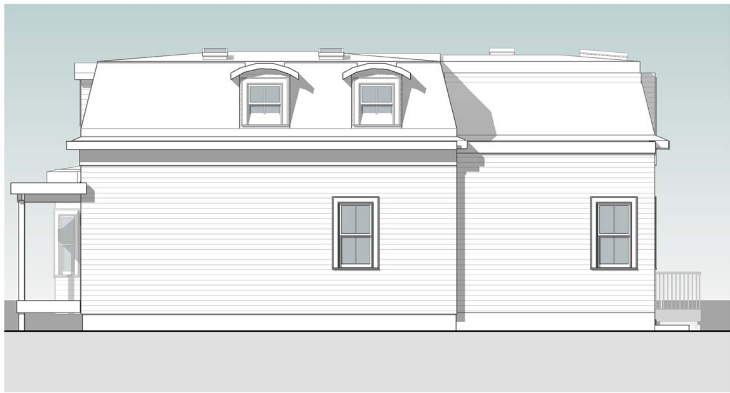
④ RIGHT ELEVATION - FRONT HOUSE 1/8" = 1'-0"
