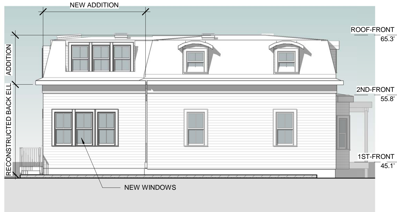
② LEFT ELEVATION - FRONT HOUSE 1/8" = 1'-0"
