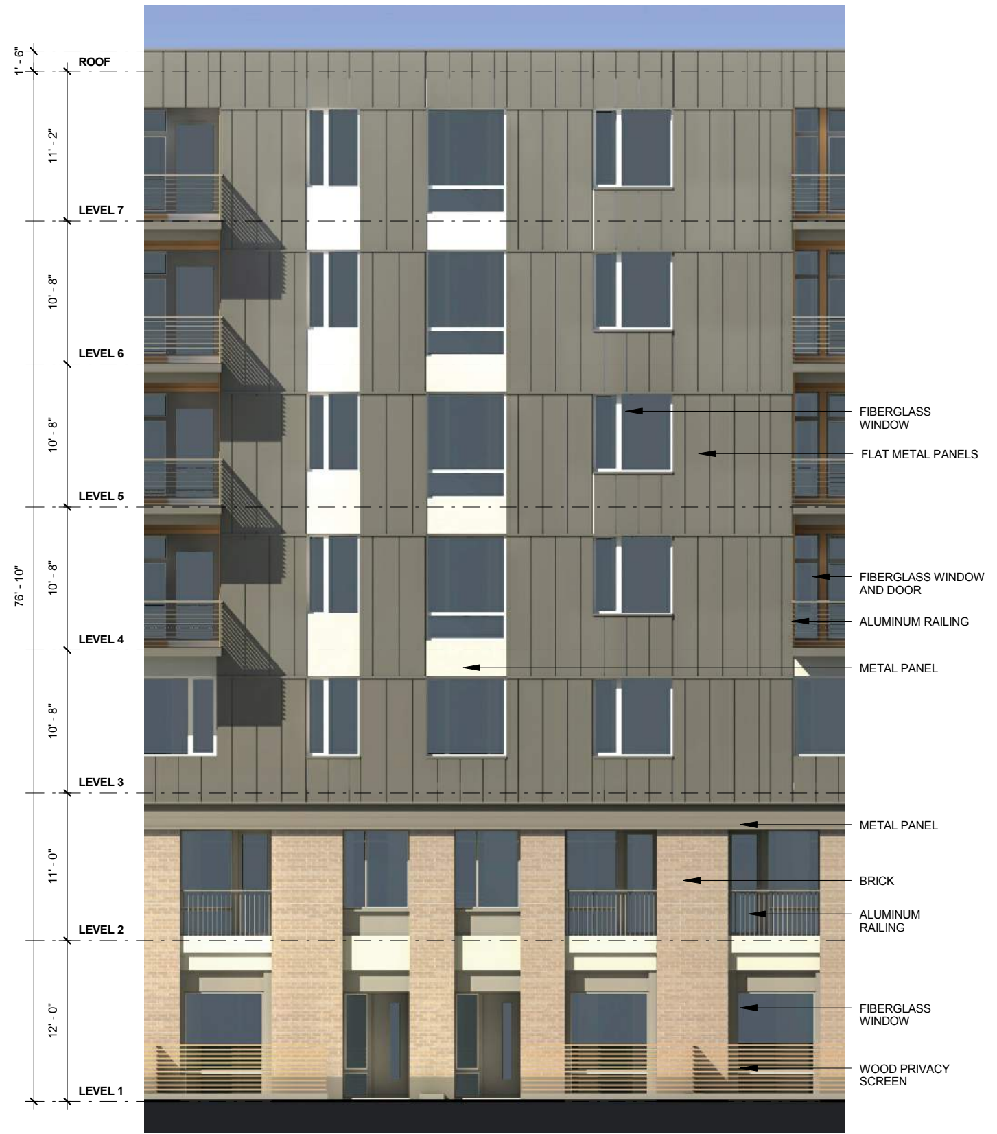
B BUILDING 1 NORTH (MEWS) PARTIAL ELEVATION
