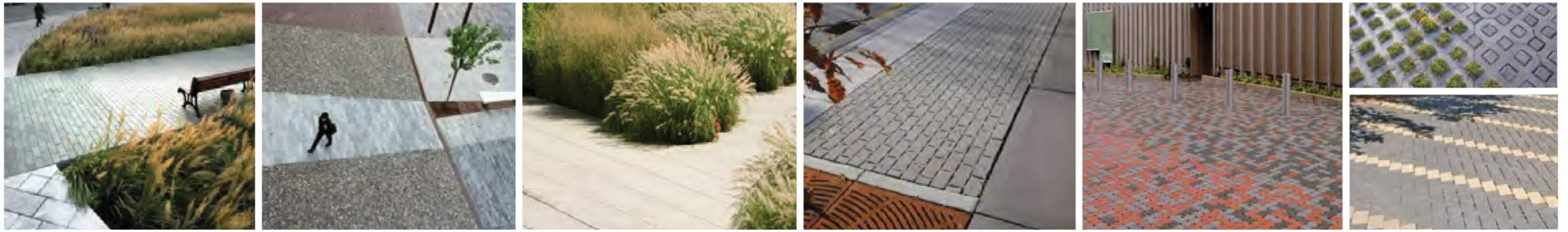
UNIT PAVERS- TEXTURAL VARIATION FOR SPEED CONTROL AND VISUAL ORIENTATION
