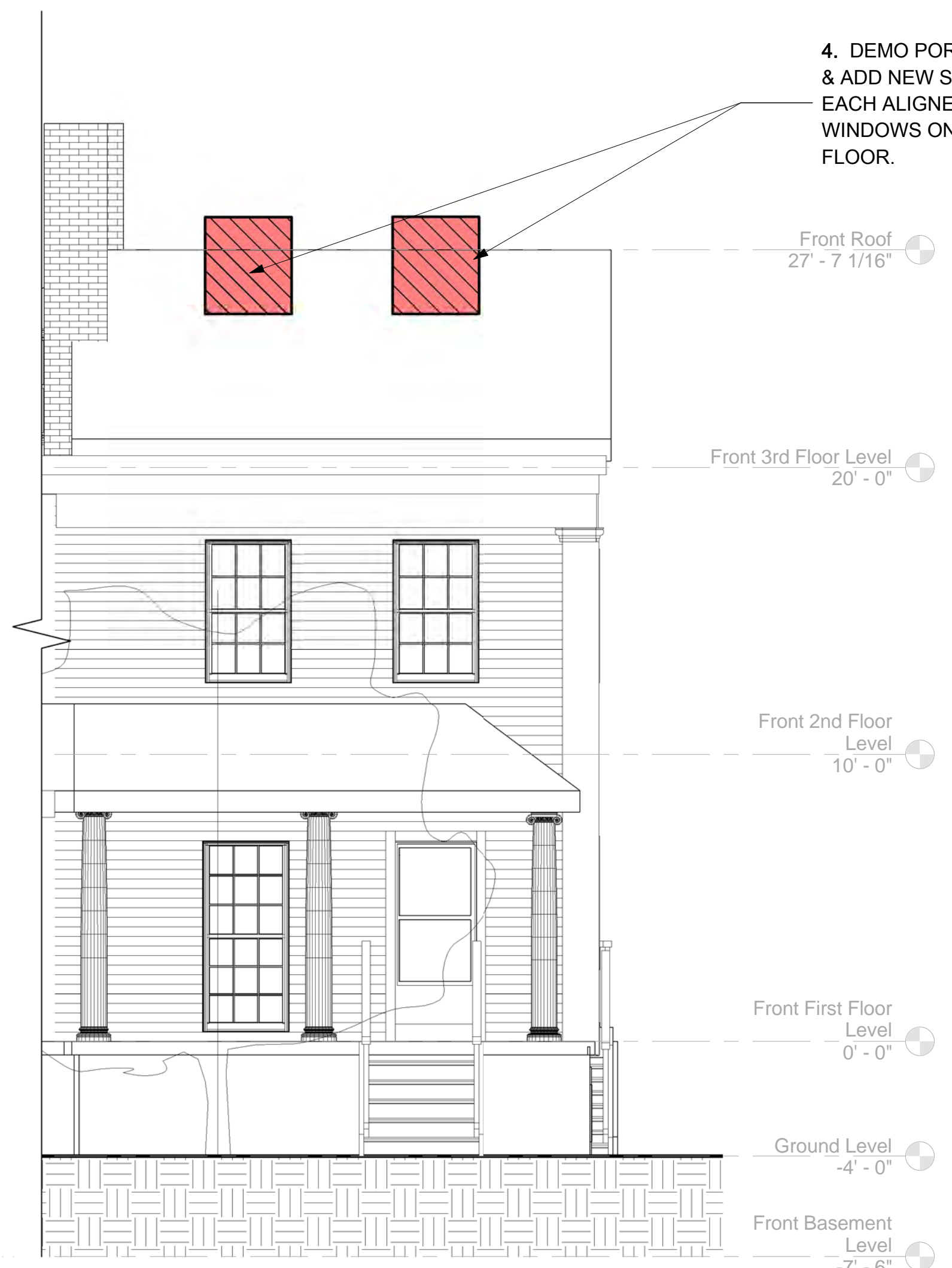
Existing Single Family-Inman Street Elevation 1/4" = 1'-0"
