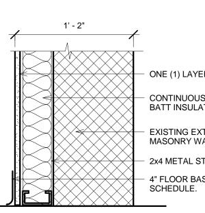
EXISTING EXTERIOR MASONRY WALL - 2x4 METAL STUDS @ 16" O.C. 4" FLOOR BASE PER FINISH SCHEDULE.
