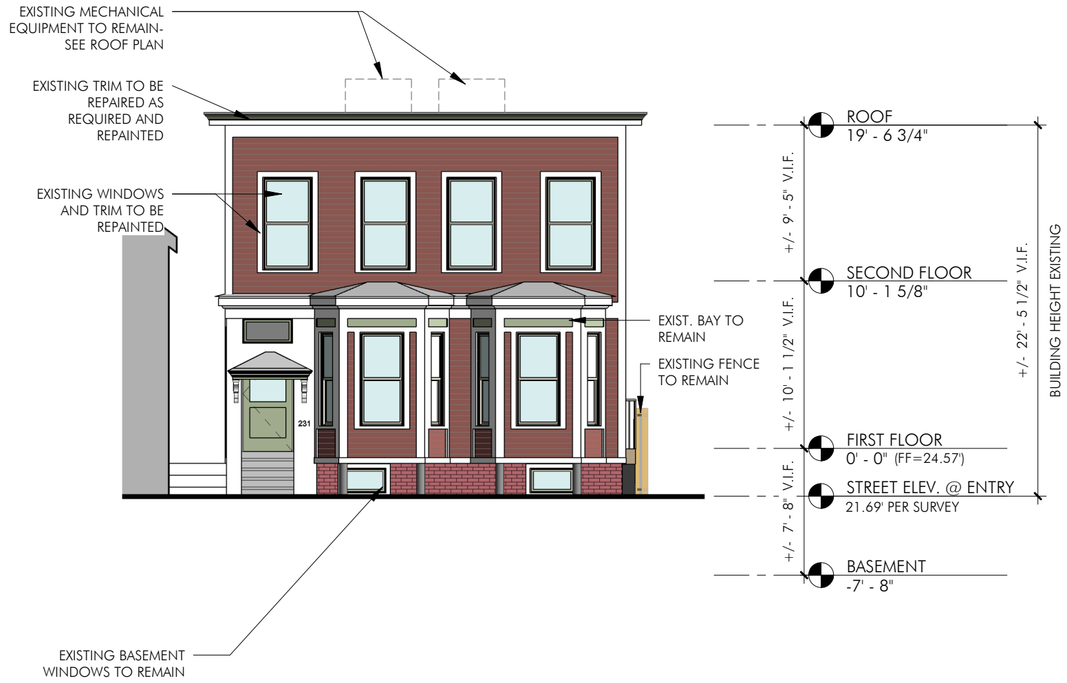
1 FRONT (EAST) EXISTING ELEVATION 1/8" = 1'-0"
