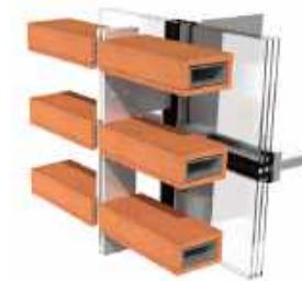
⑧ Integrated Horizontal Sun Shade at Curtain Wall with Ultra High Performance Concrete or Custom Finished Metal to Match Accent Panel Color
