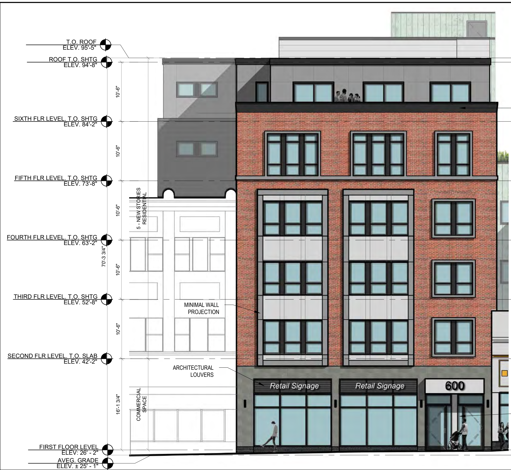
① MASS AVE ELEVATION (FRONT) SCALE: 1/8" = 1' - 0"
