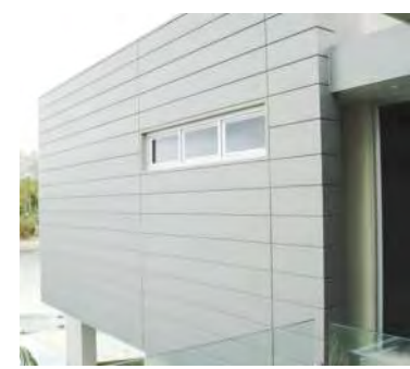
9 METAL SIDING- HORIZONTAL- LIGHT GRAY
