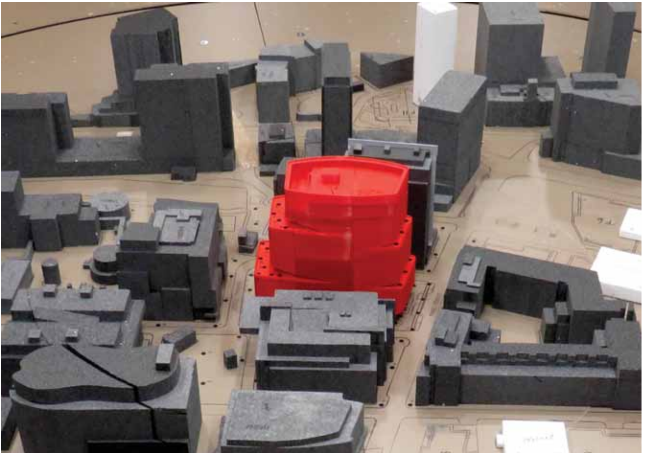
Image 2B: Wind Tunnel Study Model – Build Configuration
