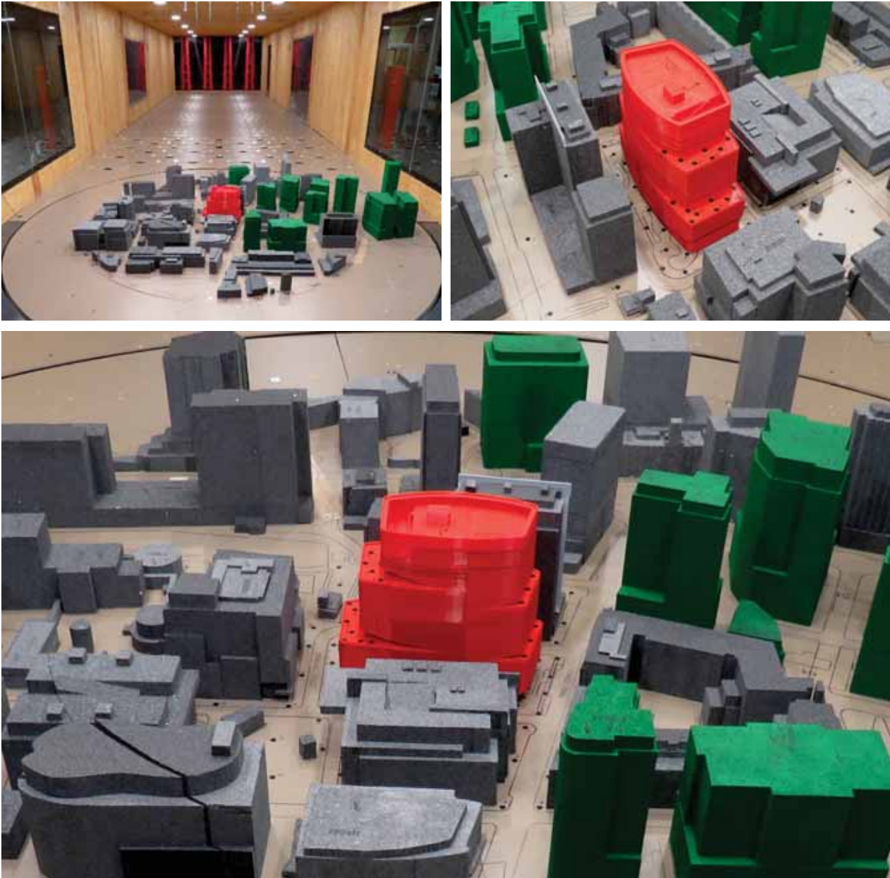
Image 2C: Wind Tunnel Study Model – Full Build Configuration
