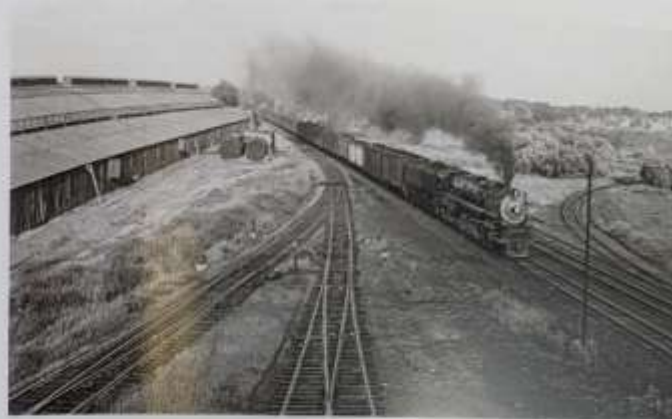
Class R-1 4-B-2 4115 (Baldwin, 1941) was leading freight 2843 (Boston to Mechanicsville, N.Y.) on the Fitchburg main line on June 15, 1942. The view is east from the Alewife Brook Parkway overpass, in the left foreground is the connection between the Central Mass. and Lexington Branches. The tracks in the center foreground led to the West Cambridge freight yard. The New England Brick Co. is on the far left and the west leg of the wye connection to the Waterbury Branch is on the far right. Albert G. Hale, WTC
