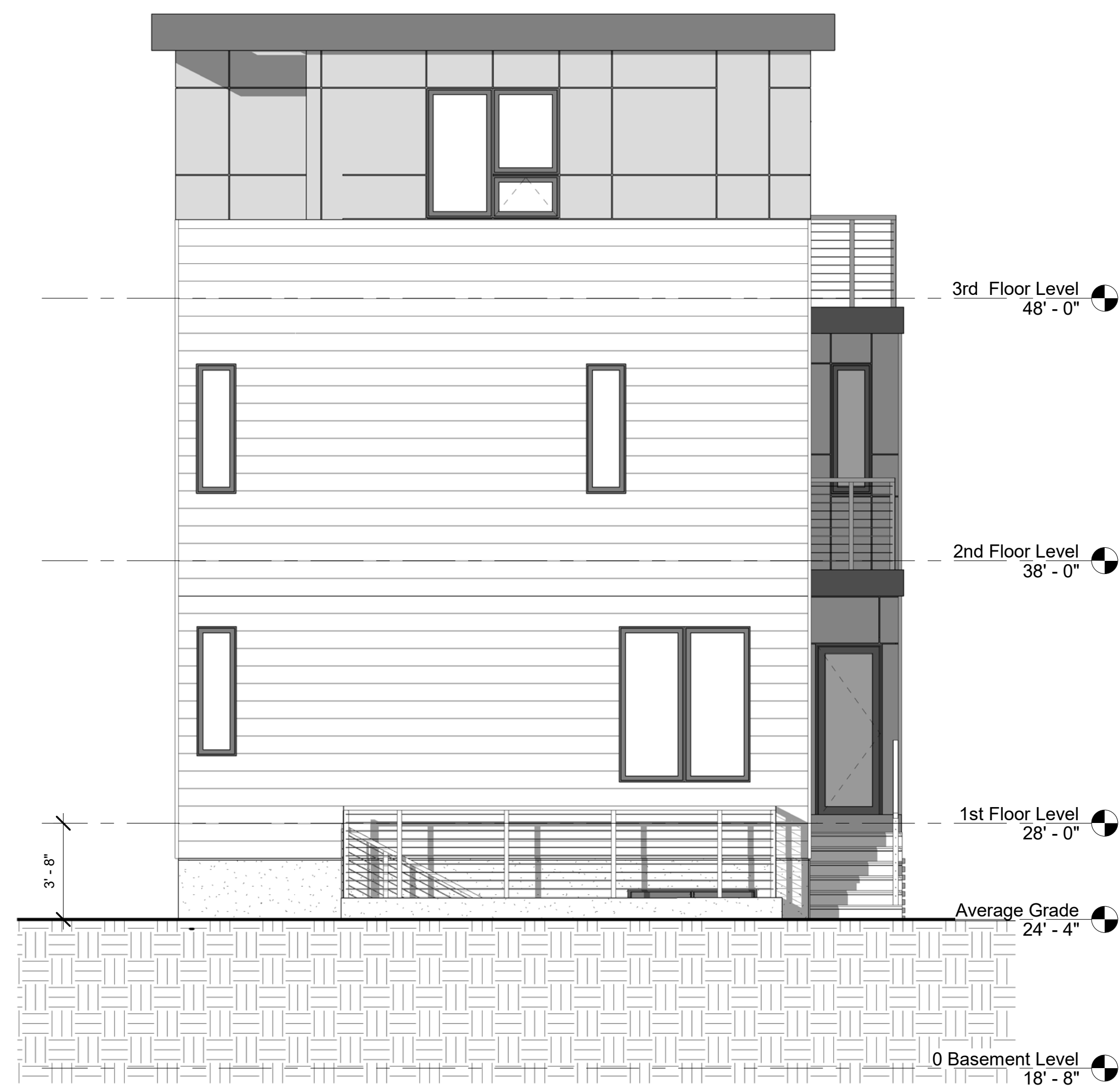
① East Elevation - Unit #1 1/4" = 1'-0"
