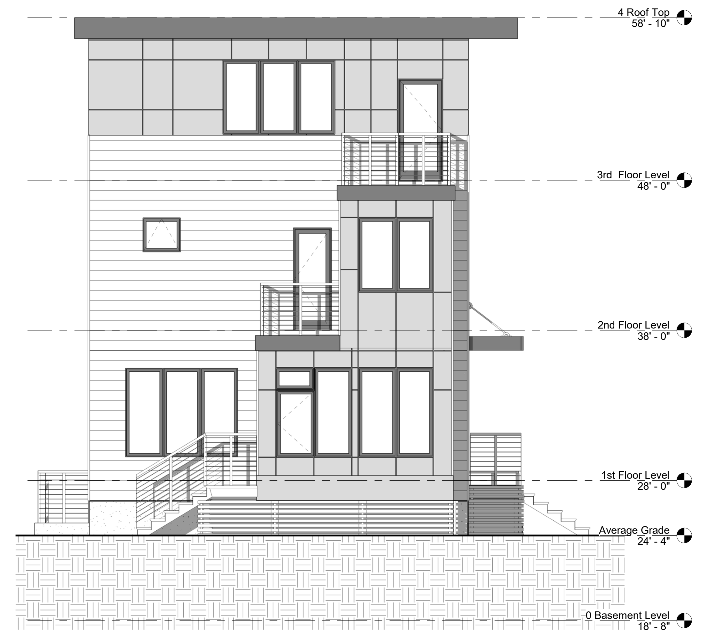
② North Elevation - Unit #1 1/4" = 1'-0"
