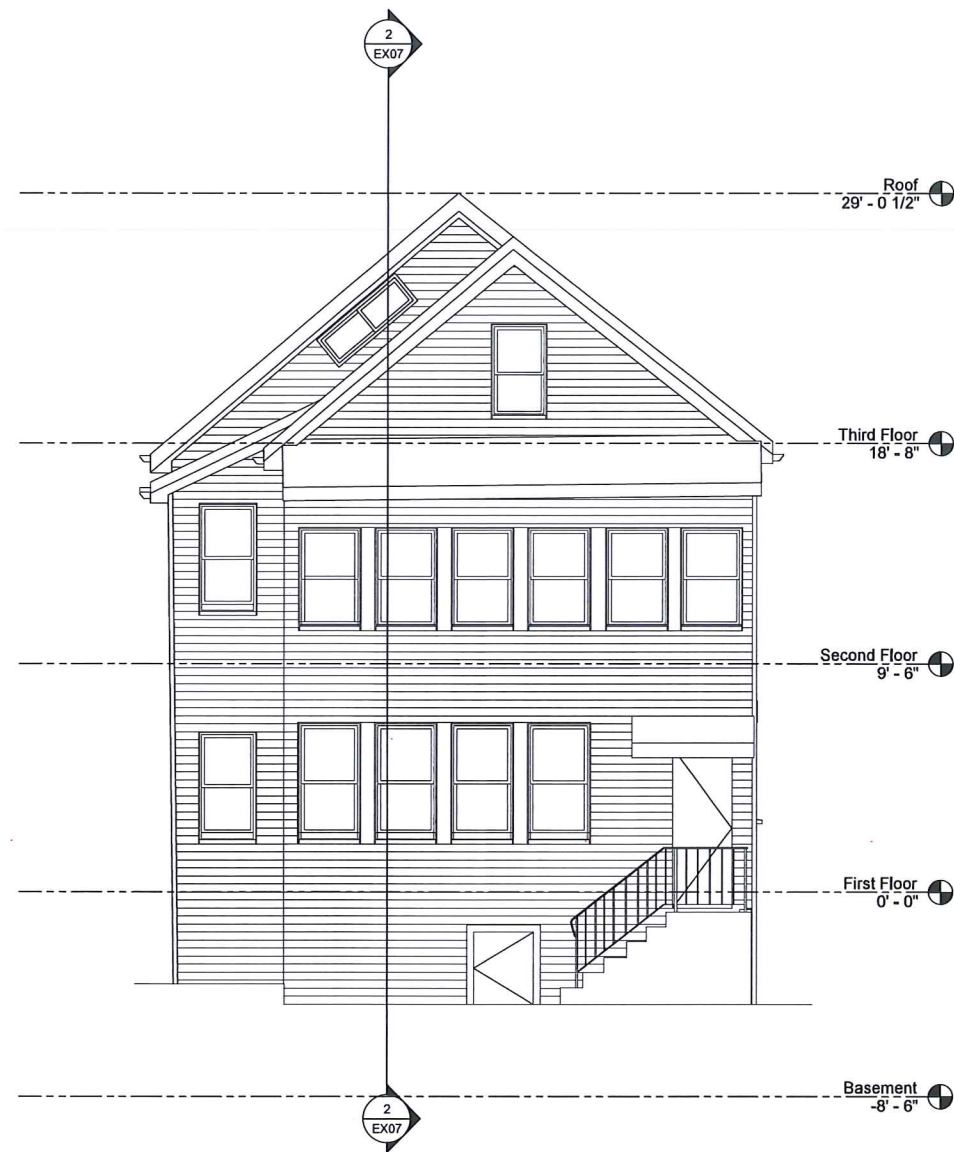
EXISTING REAR ELEVATION
