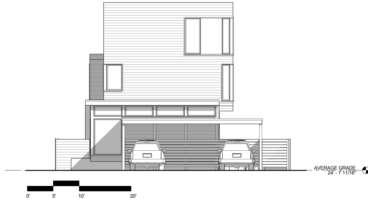
② West Elevation from Murdock Street 3/32" = 1'-0"
