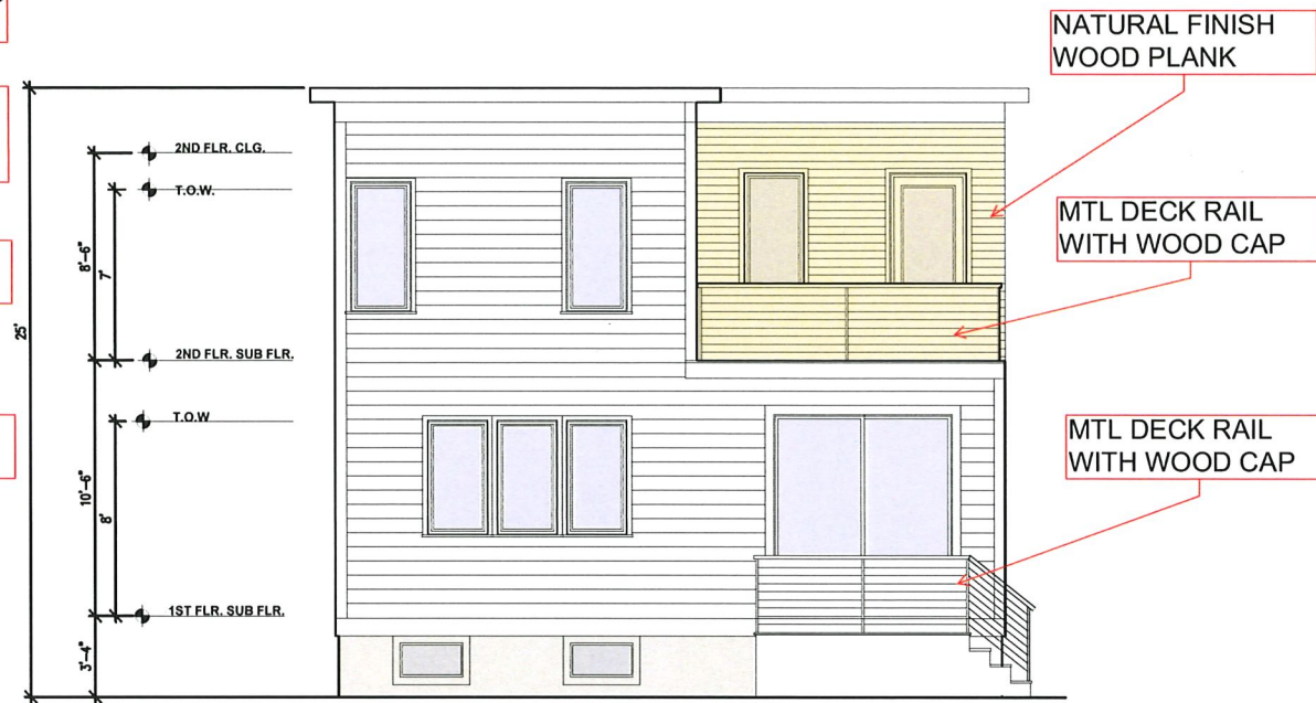
2 ELEVATION: EAST A2.1 Scale 1/4" = 1'-0"
