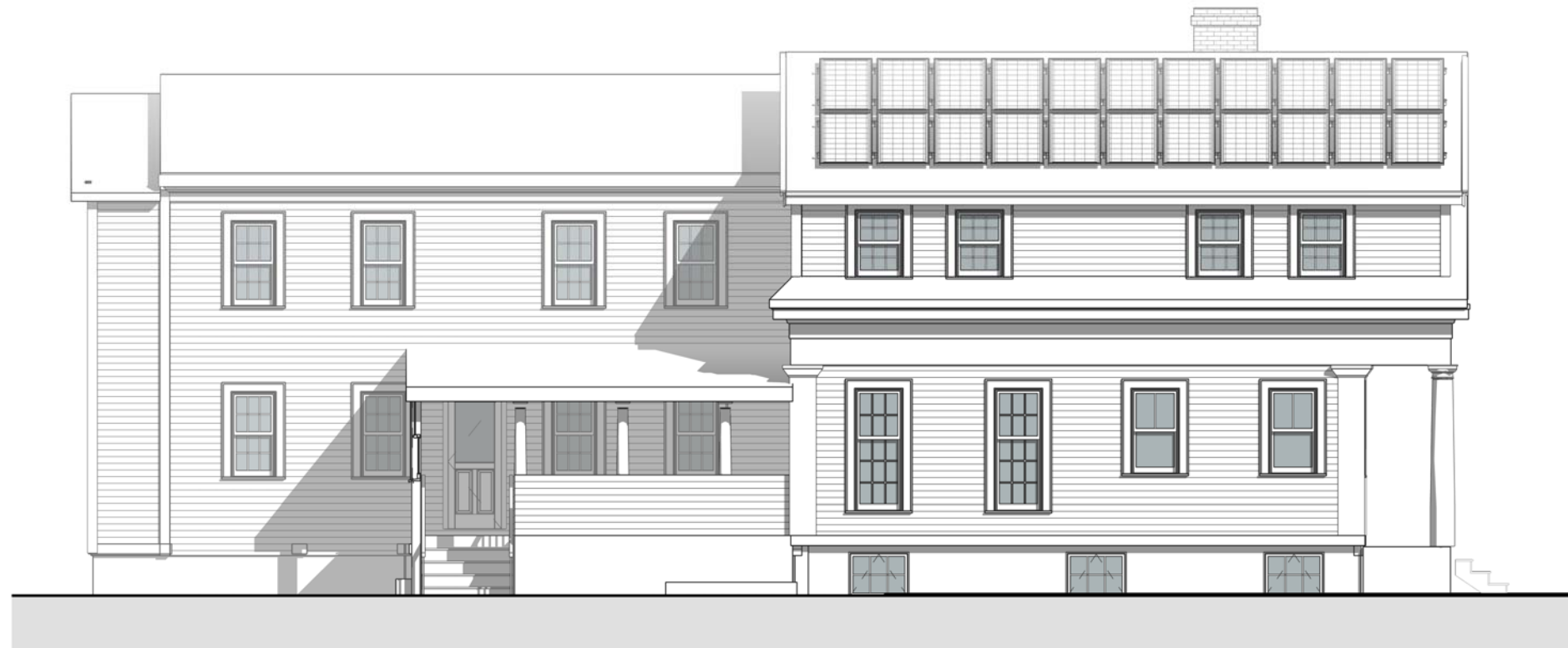
① EXISTING LEFT ELEVATION 1/8" = 1'-0"
