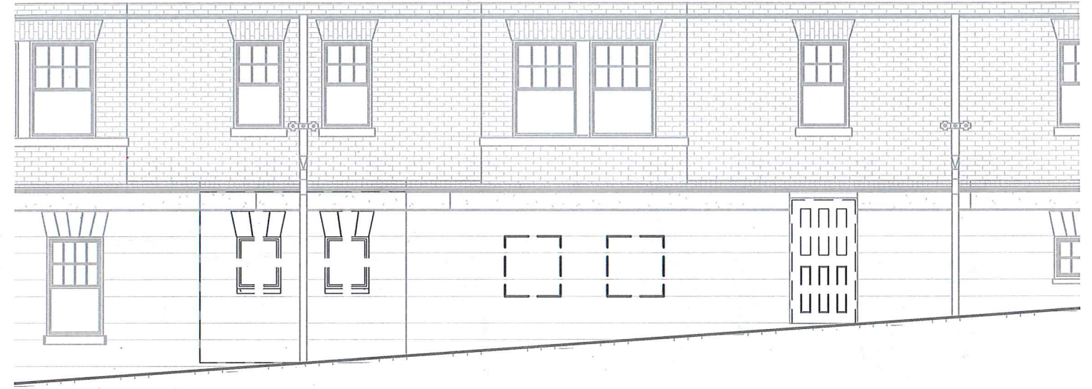
EXISTING ELEVATION - EXISTING ENTRY, BLANK WALL, AND PAIR OF FIXED WINDOWS
