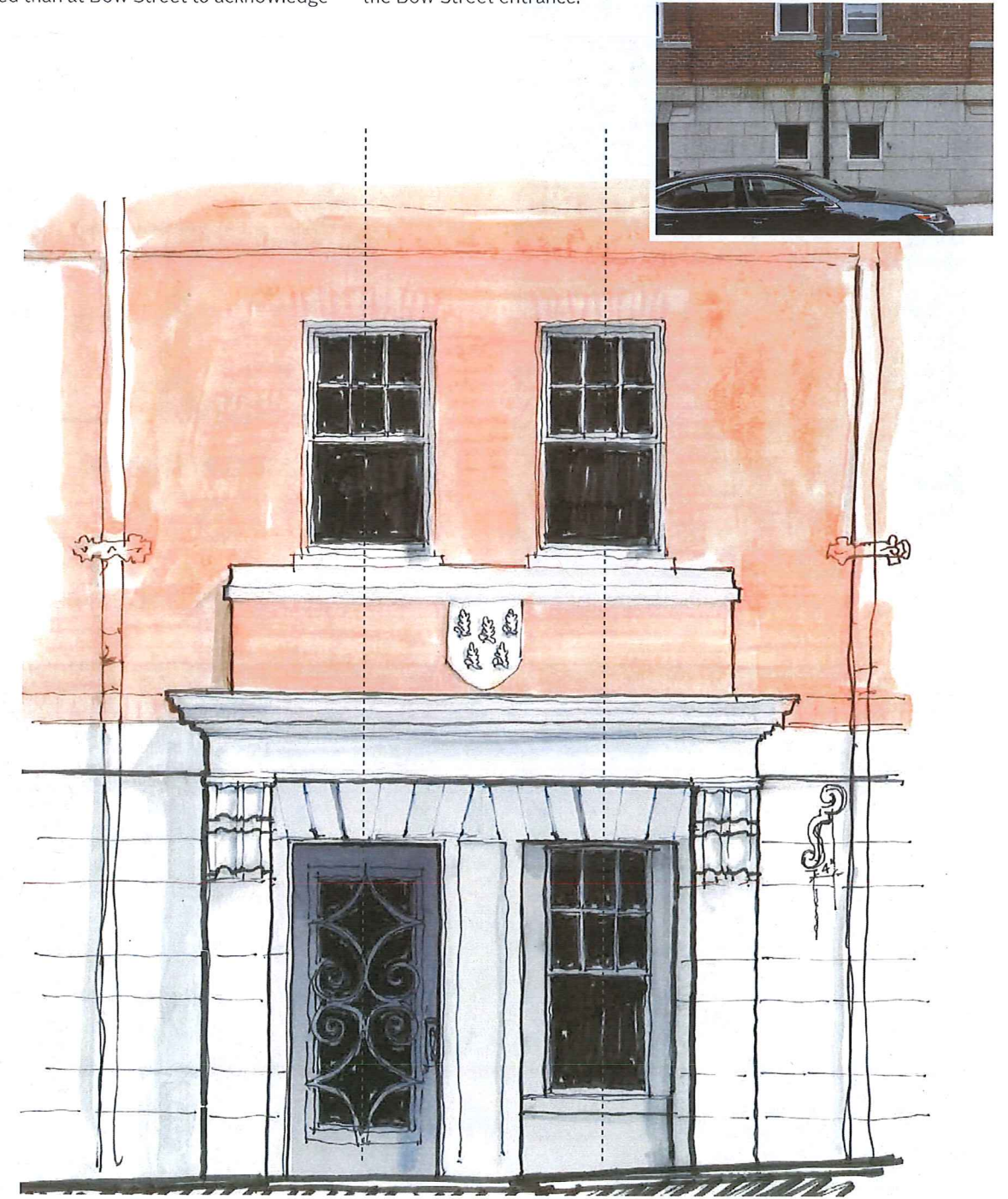
PROPOSED ELEVATION - ACCESSIBLE MID-BLOCK ENTRY ON PLYMPTON
