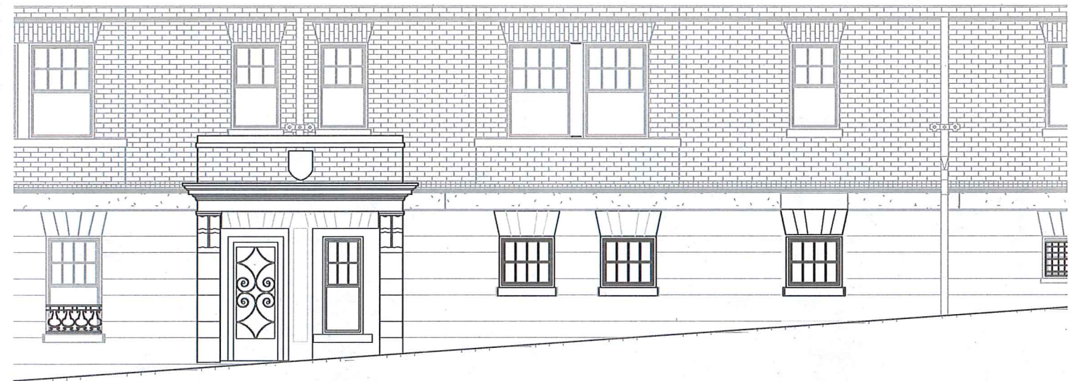
PROPOSED ELEVATION - NEW ENTRY, TWO NEW WINDOWS, AND DOOR CONVERTED TO WINDOW
