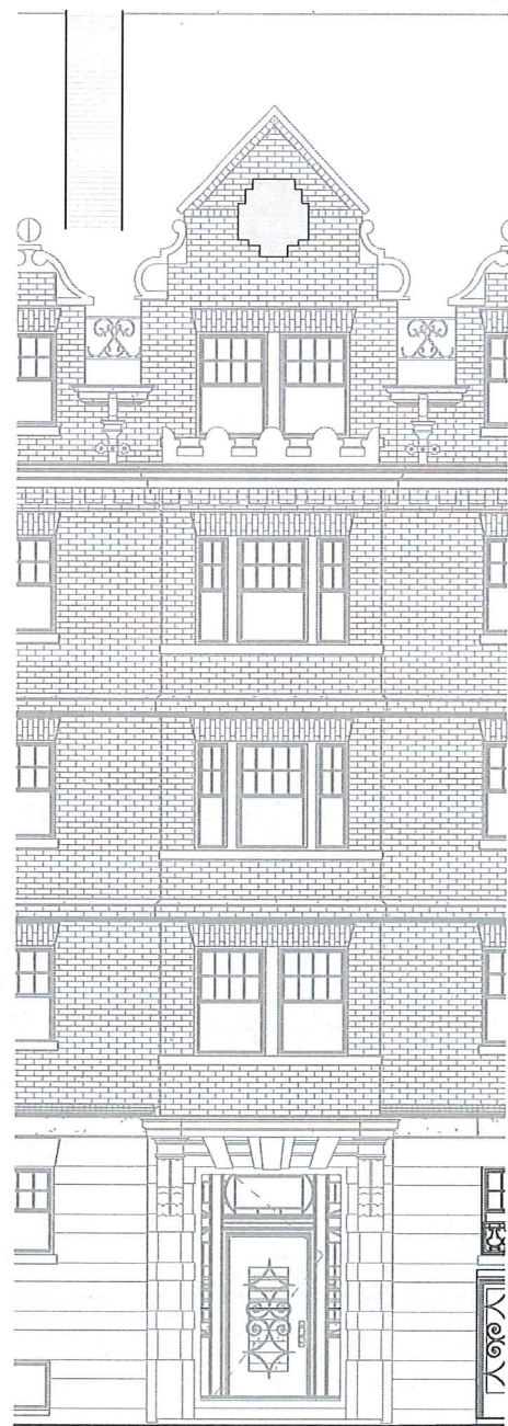
EXISTING BOW ST ENTRY PORTAL CENTERED UNDER PRIMARY GABLE
