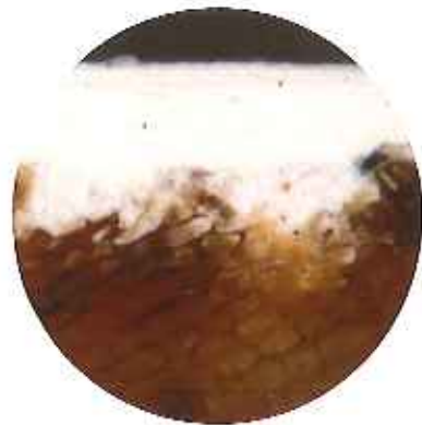
wood ceiling cross section photomicrograph 100x magnification
