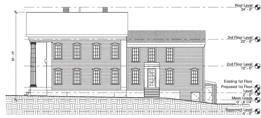
5 Existing Right Side Elevation 1/8" = 1'-0"
