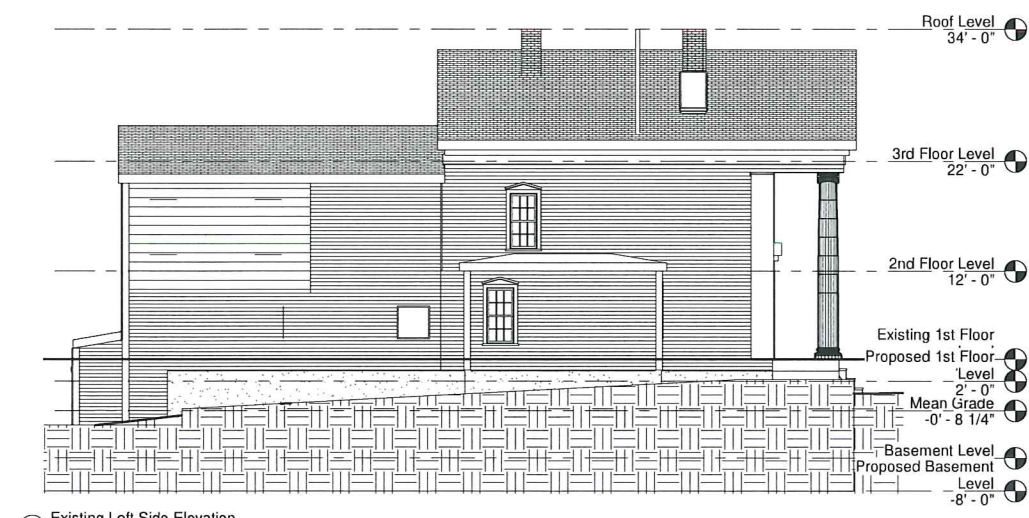
8 Existing Left Side Elevation 1/8" = 1'-0"
