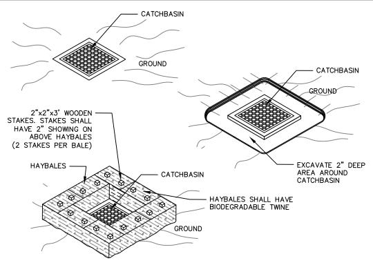
INSPECTION SCHEDULE SHALL COMPLY WITH THE 2008 EPA CONSTRUCTION GENERAL PERMIT THIS METHOD OF INLET PROTECTION IS APPLICABLE WHERE THE INLET DRAINS A RELATIVELY FLAT AREA (SLOPE NO GREATER THAN 5%). WHERE THE INLET ACCEPTS SHEET OR OVERLAND FLOWS (NOT GREATER THAN 1 CFS). THIS METHOD SHOULD NOT APPLY TO AN INLET ACCEPTING CONCENTRATED FLOW.
