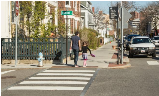
EXAMPLE OF RAISED SIDE STREET TREATMENT
