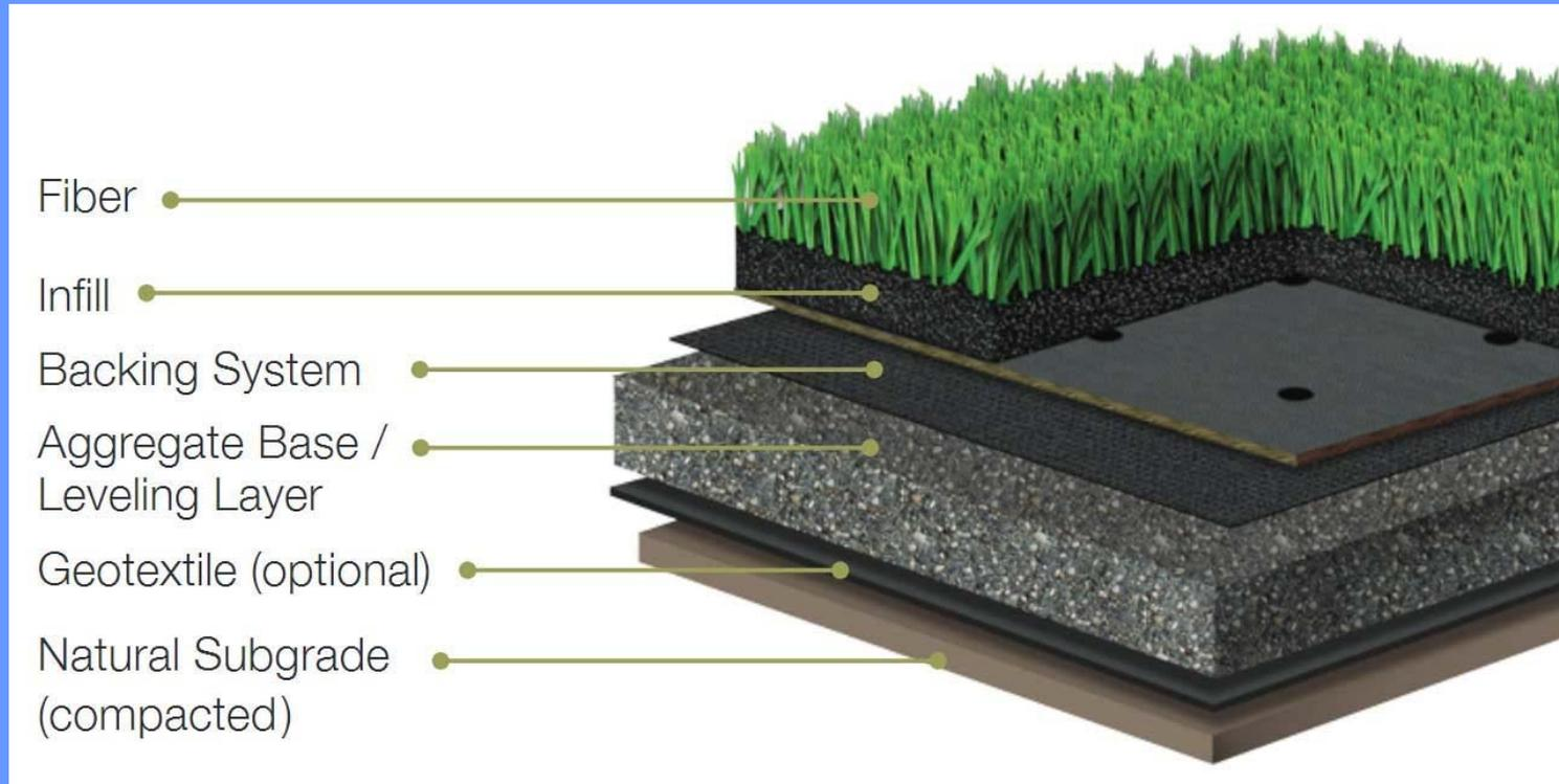
Proposed System: 2.5" fiber with Sand and Virgin EPDM Rubber Infill
